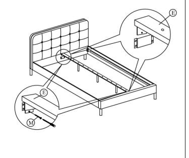
Step 5: Tighten all the 4 corner ,follow by assembly of the slat holders with LVL slats as shown.  $\bigcirc$
